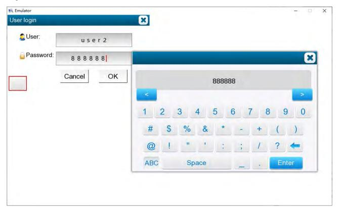
Step 6. Return to basic window 1, click the numeric value input component, system prompts "Access denied".
