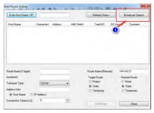
Step 5. Select the device whose Host Name starts with "CX" in the list, select **IP Address**, configure relevant parameters, and click **Add Route**.
